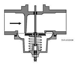
These valves are of the normally closed one-way high-flow types. The swing-type flap has no profile.
