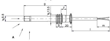
QRB1...W... with connector AGK56.38 and strain relief AGK68...
