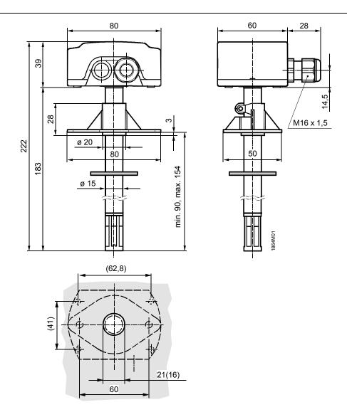
Drilling plan with (without) mounting flange
