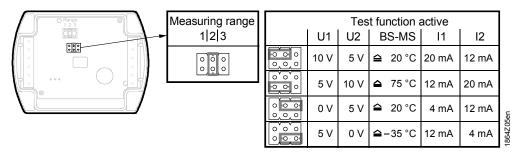
The setting element is located inside the cover. It comprises 6 pins and a jumper. It is used to select the required measuring range and to activate the test function.
