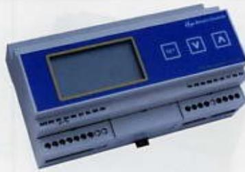
The E14 Temperature controller is a fully digital controller which can be configured with 1, 2 or 3 0-10VDC outputs and other optional features such as proportional + integral control and low limit. Night setback is standard (time switch not provided).
